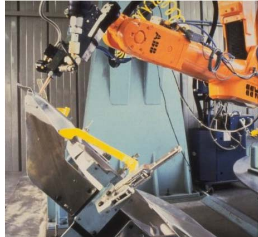
Vehicle manufacture using an epoxy adhesive. Here, vehicle - robotically delivered single-part heat-curable epoxy adhesive
