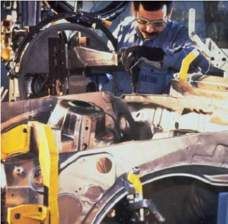
Volvo vehicle joined using adhesives. A Volvo vehicle is joined by adhesives using a proportional adhesive dispenser
